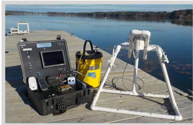
Figure C1 - Underwater HD Seaviewer Camera with PVC frame used to ground truth bottom type.
