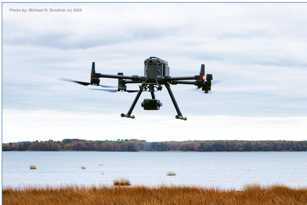
Figure 2 – Photo of the DJI Matrice 300 Drone in flight on its way to survey the southeastern section of Great Bay. (Photo by Michael R. Routhier).
